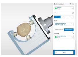
Milling mode: fast - to have more time for postprocessing. Material: Katana Zirconia STML A3.
